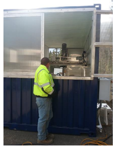
Industrial composter at Grand Portage transfer station
